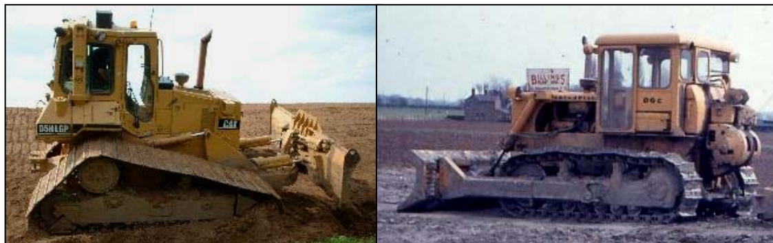
Left; a “hi-track” bulldozer. Right; amore traditional flat- tracked machine
